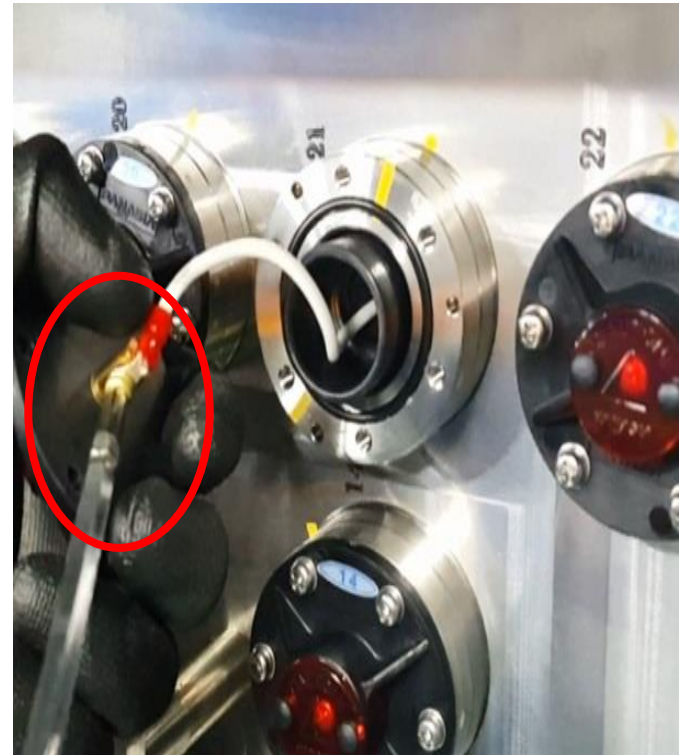
Unscrew bolts connected with the UV lamp wires
