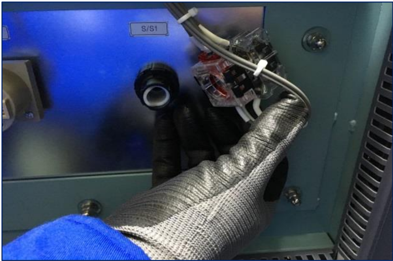
Check and replace the Select Switch
