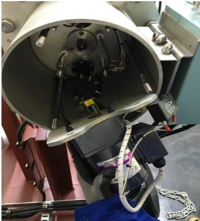
Dismount Wiper Motor and Coupling
